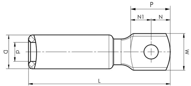
Al terminal for stranded Al cable 150 mm<sup>2</sup>, or for solid Al cable 185 mm<sup>2</sup> with an M16 hole in the palm. Used with Elpress certified systems V1300 or V250.
